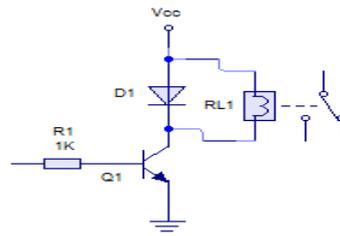
Figure 5: Transistor Switch Driver
