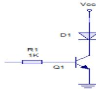
Figure 3: Transistor Switch
